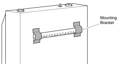
Figure 6 - Mounting Bracket Location
